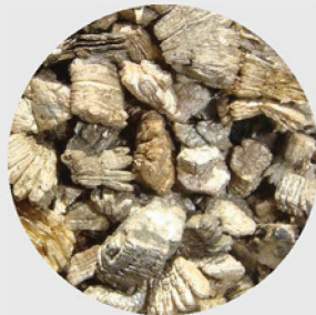
Asbestos Contaminated Vermiculite
